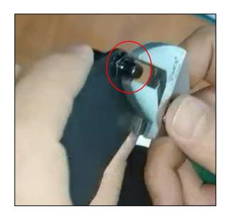
18. Align the rotating shaft with the mounting hole of the refrigeration door, open the door 170 degrees, and fix the middle hinge seat with 2 screws
