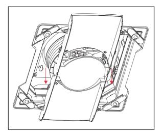
• Pull the air duct down until it engages with the plenum mounting bracket. The duct connects to the bracket with four catches that will clicks when secure.
