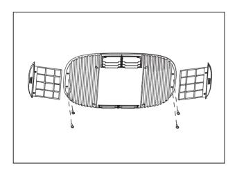
• Finally, fit both return air filters into the plenum properly and the **installation is all completed**.
