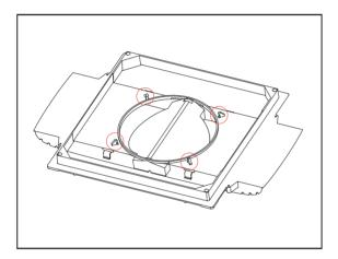
• When you have heard 4 clicks and the end of the duct is firmly parallel to the top side of the bracket then you have successfully connected.
