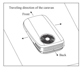
• There shall be a space of 100mm/4" minimum all around the roof top unit to ensure suitable air flow and access for maintenance.
