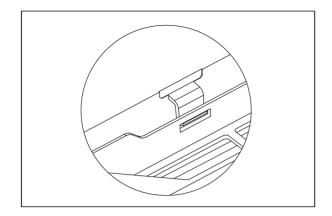
• Fix the plenum assembly on the plenum mounting bracket with four ST4.2×19 pan head screws.
