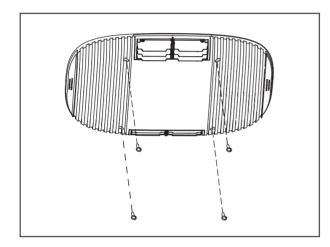
• Take out the return air filters and fix the plenum to the ceiling with 4 provided countersunk head screws.
