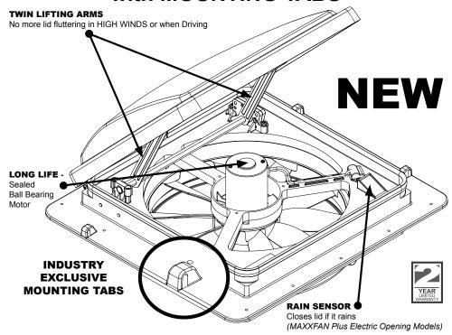
**INDUSTRY EXCLUSIVE BUILT-IN waterproof molded mounting tabs** allow for **FAST** and **TOOL-FREE INSTALLATION** of optional **MAXXAIR FANMATE** cover (sold separately).
